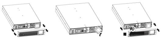
Figure 3-4 Tower-mounting the UPS
